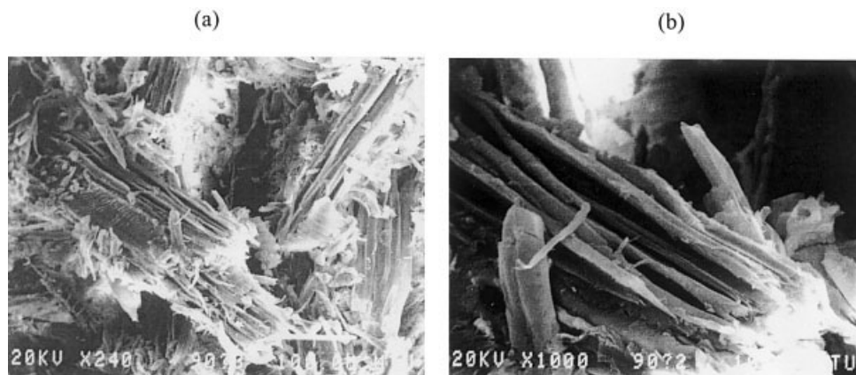
Figure 2 SEM micrographs of sugar maple wood flour at (a) \times 240 magnification and at (b) \times 1000 magnification.
